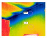
Reduced insulation effectiveness at cavity head / eaves junction
